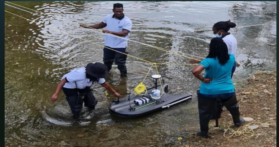
River Discharge Measurement using a river surveyor – Water Resource Agency
